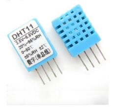
The DHT11 is a basic, low-cost digital temperature and humidity sensor. It uses a capacitive humidity sensor and a thermistor to measure the surrounding air, and interface is a digital signal on the data pin (no analog input pins needed). It's fairly simple to use, but 9requires careful timing to grab data. The only real downside of this sensor is you can only get new data from it once every 2 seconds, so when using our library, sensor readings can be up to 2 seconds old.
