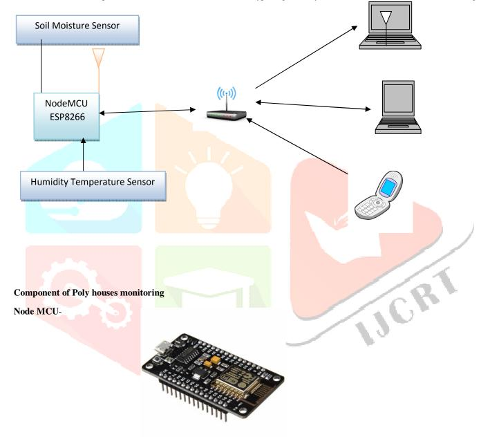
NodeMCU is an open source IoT platform. It includes firmware which runs on the ESP8266 Wi-Fi SoC from Espressif Systems, and hardware which is based on the ESP-12 module. The term "NodeMCU" by default refers to the firmware rather than the dev kits. ... It uses many open source projects, such as lua-cjson, and spiffs.
