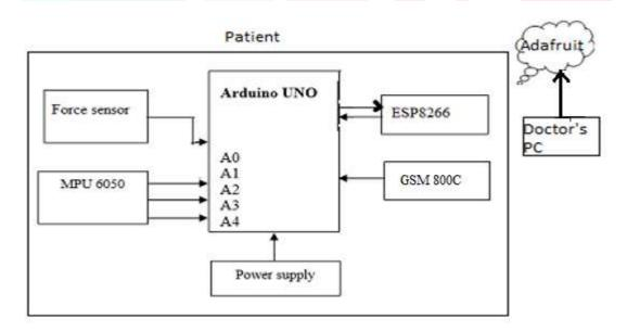
Figure 3.1: Block diagram for proposed system
