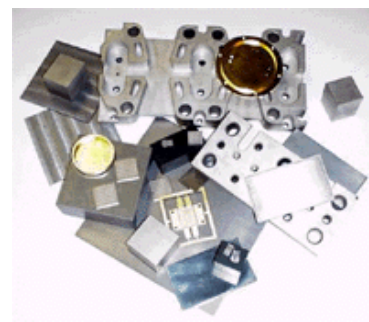
Figure 5. Discontinuously reinforced aluminum MMCs for electronic packaging applications: (a-top) \text{SiC}_p/\text{Al} electronic package for a remote power controller (photo courtesy of Lockheed Martin Corporation), and (b-bottom) cast \text{Gr}_p/\text{Al} components (photo courtesy of MMCC, Inc.).
