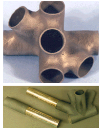
Figure 4. Cast \text{SiC}_p/\text{Al} attachment fittings: (a-top) multi-inlet fitting for a truss node, and (b-bottom) cast fitting brazed to a Gr/Al tube.
