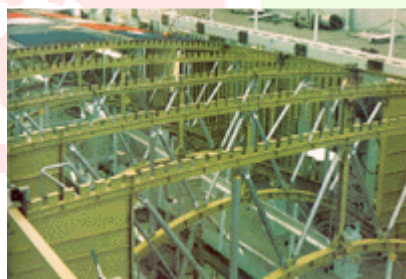
Figure 1. Mid-fuselage structure of Space Shuttle Orbiter showing boron-aluminum tubes. (Photo courtesy of U.S. Air Force/NASA).
