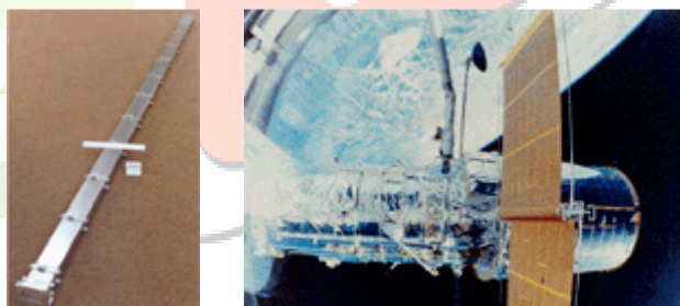
Figure 2. The P100/6061 Al high-gain antenna wave guides/ boom for the Hubble Space Telescope (HST) shown (a-left) before integration in the HST, and (b-right) on the HST as it is deployed in low-earth orbit from the space shuttle orbiter.
