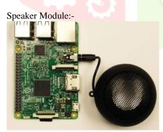
The speaker module is used to get audio output. The speaker module is connected to raspberry pi to get audio output.
