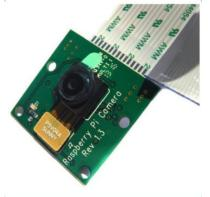
The camera consists of a small circuit board ,which connects to raspberry pi's camera serial interface bus connector via a flexible ribbon cable. The camera module takes high definition video as well as photographs.
