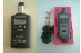
Figure 4 Hygrometer and Moisture meter
