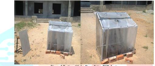
Figure 5 Testing of Solar Dryer Using POP sheets
