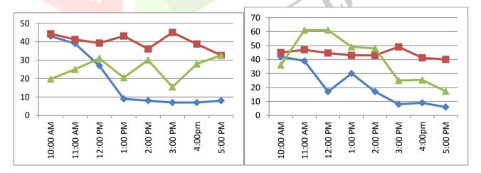
We have observed that more heat is losing from the back side of the drier i.e., from steel sheet.
