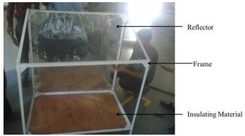
Figure 1 Design of Solar Dryer Equipment
