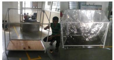
Figure 3 Fabricated Solar Dryer
