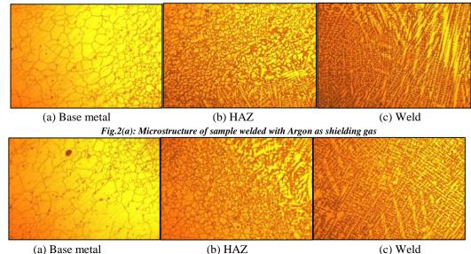
Fig.2(b): Microstructure of sample welded with Argon-hydrogen as shielding gas
