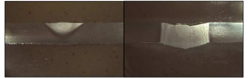
Fig 3. Macrostructure of weld (a) with Argon shielding gas (b) with Argon-Hydrogen shielding gas
