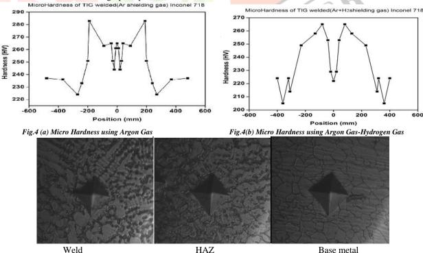
Fig 5: (a)Indentation by vicker's hardness tester on Ar welded samples.
