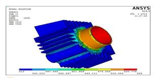
Fig. 13. Temperature Distribution through Rectangular fin3mm thickness)
