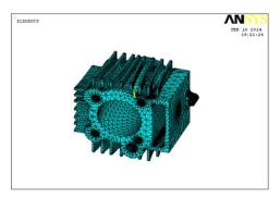
Fig.6.Mesh model of circular fin(3mm thickness)
