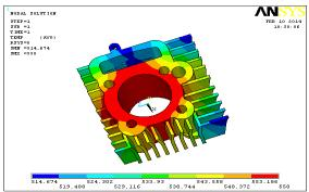
Fig.17.Temperature Distribution through curved fin3mm
