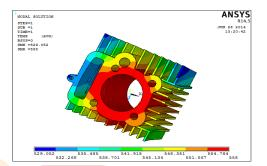
Fig.22. Temperature Distribution through curved fin 2.5mm
