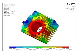
Fig.19.Temperature Distribution through curved fin 3mm
