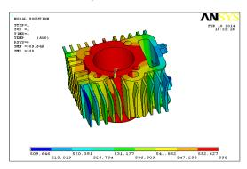
Fig. 18. Temperature Distribution through curved fin 2.5 mm
