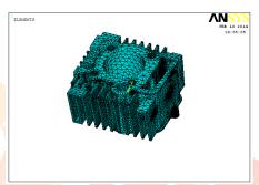
Fig.2. Mesh model of rectangular fin(3 mm thickness)
