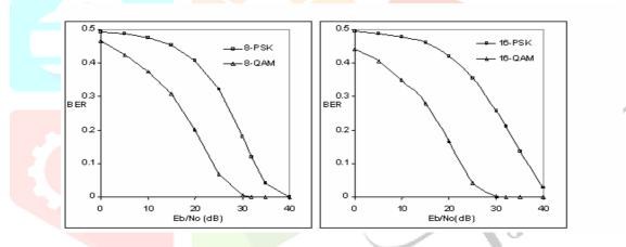
Figure 6. BER performance comparisons of 8/16-PSK and 8/16-QAM
