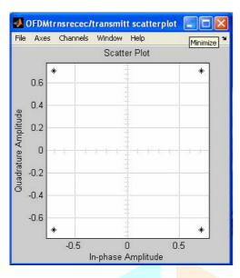
(a) Transmitted signal with 4 phases
