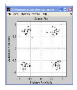
(b) Received signal with phase distortions
