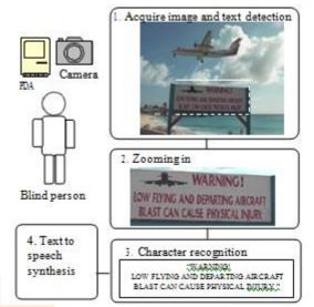
Figure 1 System configuration (walk-around mode)
