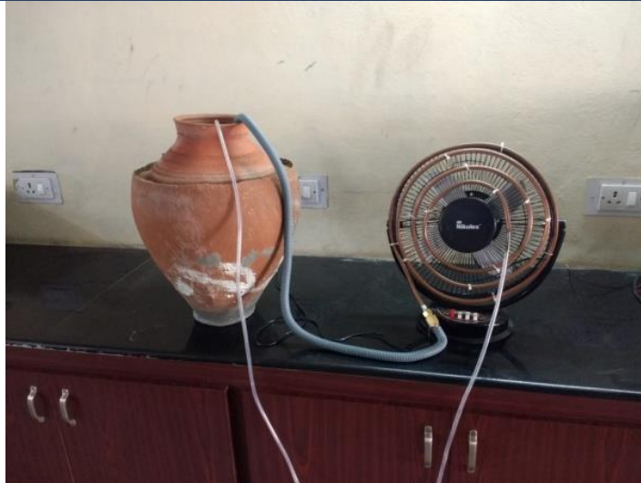
Figure 4: Representation of air cooling using zeer pot refrigeration technique
