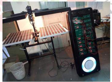
fig.8 solar PVTR system with control board connections
