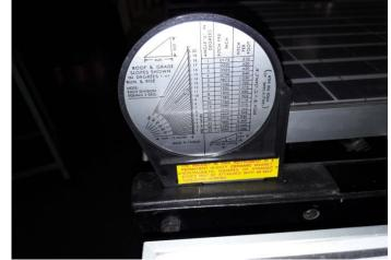
fig.9 Tilt angle indicator in solar PVTR system
