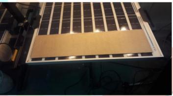
fig.7 some cells of a solar panel is shaded
