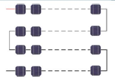
fig.3 Internal structure of the module
