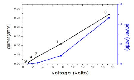
fig.5 graph showing IV and PV curves for shaded cells
