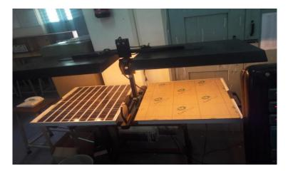
Fig.6 single panel completely shaded
