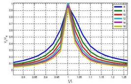
Fig. 6.2: Characteristics of SRC resonant converter
