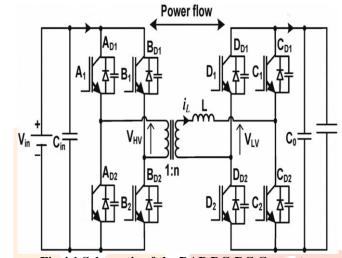
Fig 4.1 Schematic of the DAB DC-DC Converter
