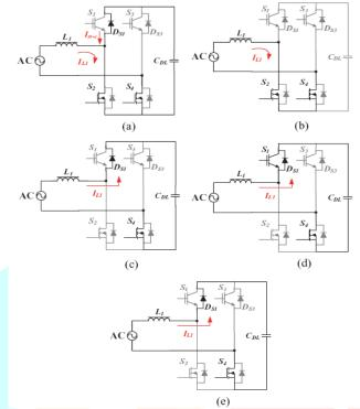
Fig.3.1 Operating modes of the proposed bidirectional ac-dc rectifier in the rectification mode: (a) *Mode* 1, (b) *Mode* 2, (c) *Mode* 3, (d) *Mode* 4, and (e) *Mode*
