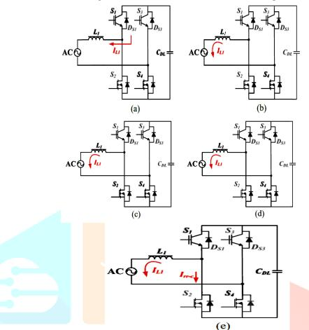
Fig. 5. Operating modes in the rectifier's generation mode using the same switching pattern as the rectification mode: (a) *Mode* 1, (b) *Mode* 2, (c) *Mode* 3, (d) *Mode* 4, and (e) *Mode* 5.
