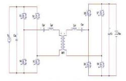
Fig 6.1 Full-bridge series resonant converter
