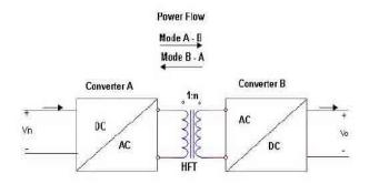
Fig. 5.2 Basic structure of isolated bidirectional AC-DC converter.
