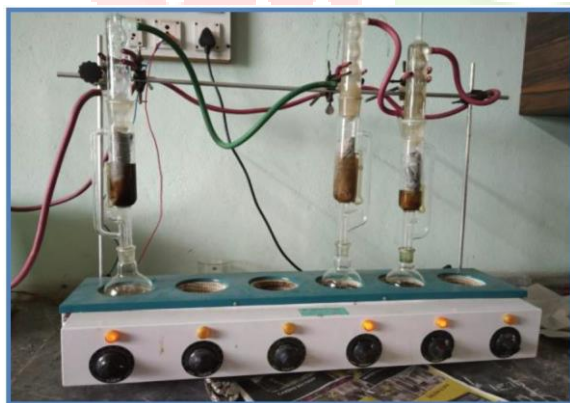
Figure 1. Soxhlet Extractor (Borosil)
