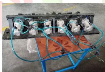
Fig 1:(fixture of mild steel under completion)
