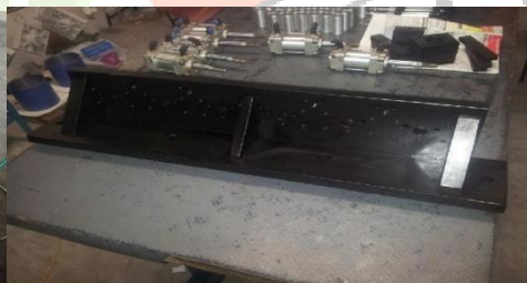
fig 2: (overall pneumatic setup of fixture) of blackening process)
