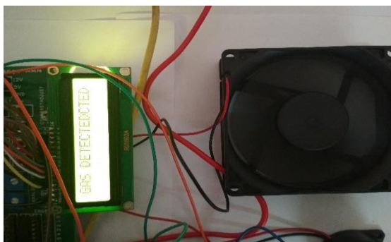
Fig.8.Test case 5-Turning of exhaust fan
