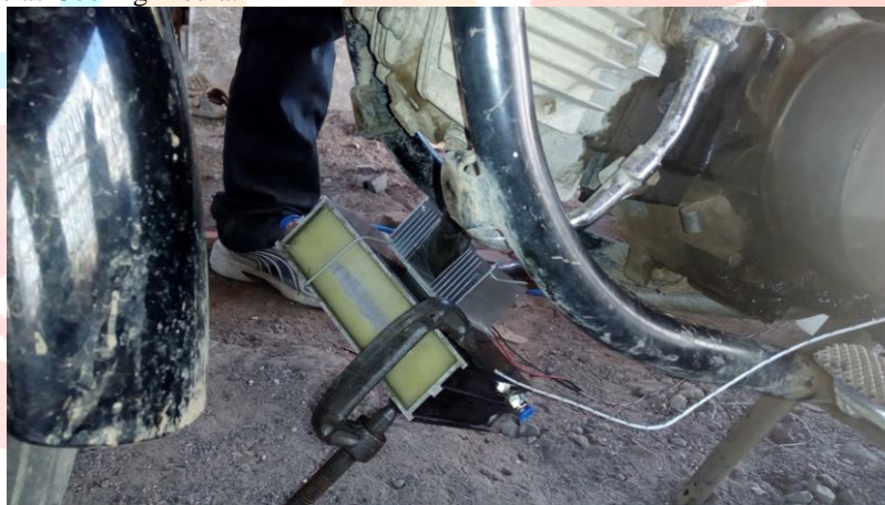
Figure 4: Water Cooling System
