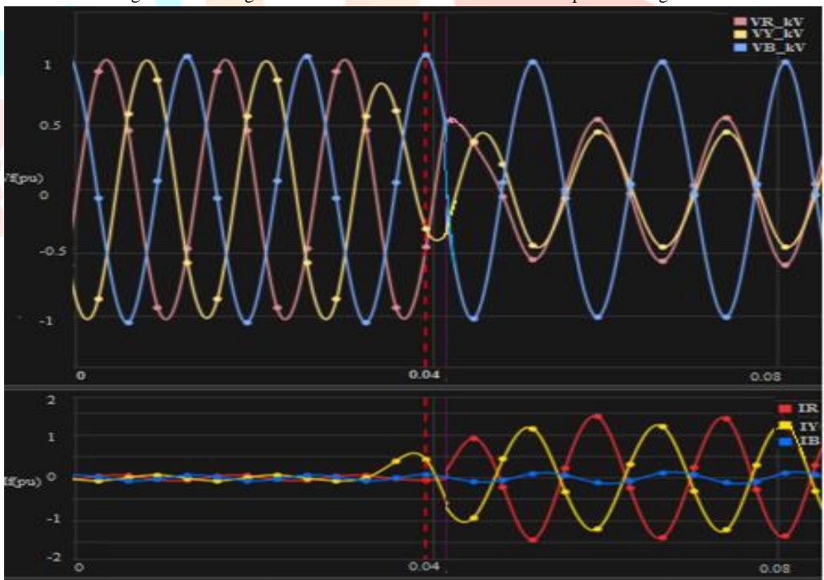
Fig.3. Fault voltage and current waveforms of LLG fault with phase R and Y to ground
