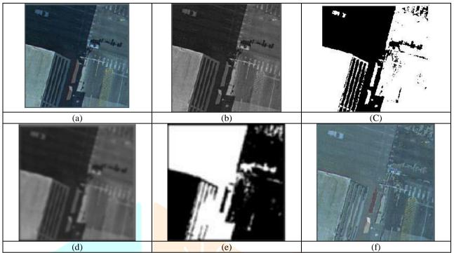
In above figure (a) Original image(b)Remove noise and convert in gray.(c) Shadow detection by our new analysis based algorithm and apply threshold .(d) Apply Gaussian filter and morphology. (e)Apply smooth masking.(f) final shadow removal for image by our new analysis based algorithm.
