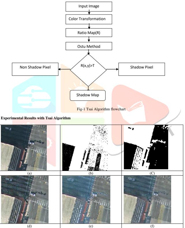
In above figure (a) Original image(b) Shadow detection by Tsai's algorithm.(c) Shadow detection by our new analysis based algorithm.(d) Shadow removal(Enhanced shadow image) using adaptive histogram equalization. (e) Shadow removal (Enhanced shadow image) using image adjustment.(f) final shadow removal for image
