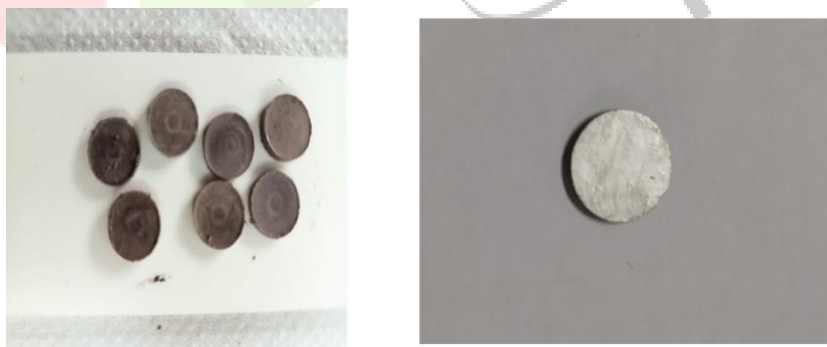
Fig. 4: Prepared BCT–CFO pellet after sintering.
