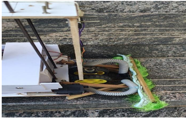
Fig 4(d) The mop touches the ground by Using servo motor to clean.
