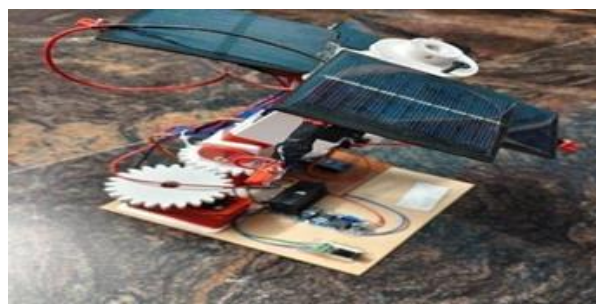
Fig 4.5 : Solar Panel Tracking System, If LDR2 > LDR4 , move Servo-1 right
