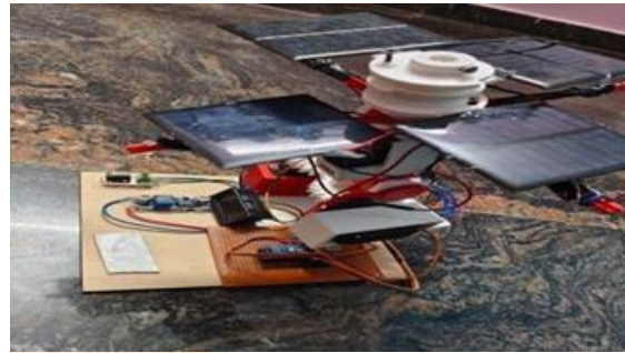
Fig 4.3 : Solar Panel Tracking System, If all LDR values \leq 500
