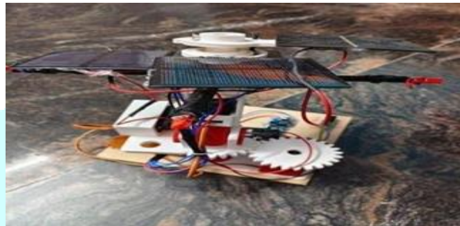
Fig 4.7 : Solar Panel Tracking System, If LDR1 > LDR3 , move Servo-2 down In Case 5 , If LDR1 > LDR3 , it means that LDR1 is detecting more light than LDR3 . Based on this condition, the system moves Servo-2 downward.
