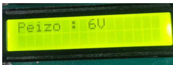
Fig 4.2 The Output voltage produced from the piezo is displayed in the LCD
