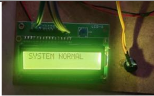
Figure 7 : LCD output when there is no abnormal activity detected
