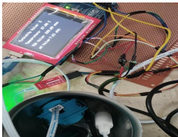
Fig 6.3 Results Of Ph Turbidity, Temperature And TDS In Fresh Water
