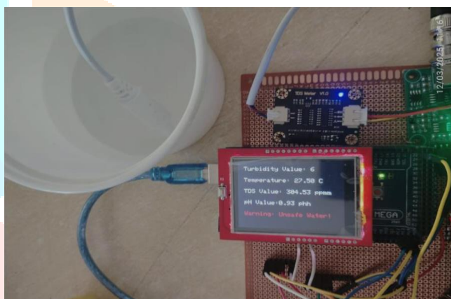
Fig 6.4 Reading Of TDS Sensor Value In Lemon Solution
