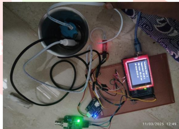
Fig 6.2 Results Of Turbidity, TDS And Temperature In Fresh Water
