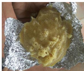
Figure 7: Adhesive used to bind wooden blocks
