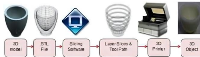
Figure 1 - 3D printing process (Adapted from [1] )
