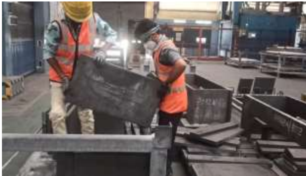
Fig. 5 Lifting and carrying of graphite board.
