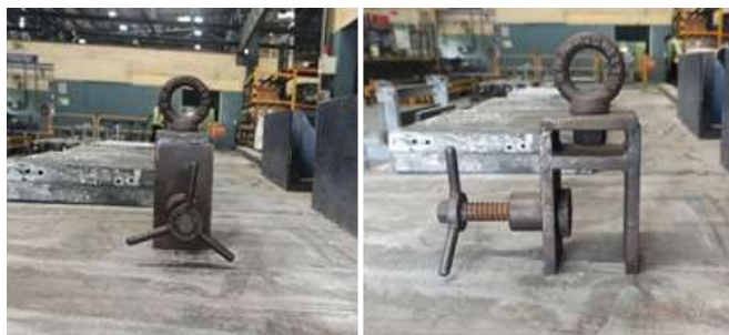
Fig. 17 Fabricated clamp for lifting and carrying.
