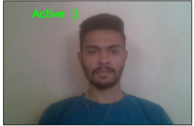
Figure 6. shows the state where the driver is fully active, and the Euclidean distance calculated is above the threshold and hence, the driver is classified into fully active state.
