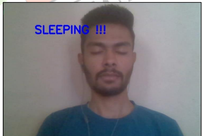
Figure 8. is a state where the driver is completely asleep, as the EAR calculated turns out to be zero, hence, falling in sleepy category.
