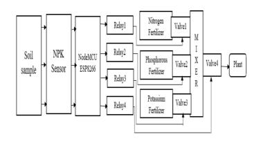
Plants are subject to a variety of environmental conditions thatvary regularly in both space and time. Soil properties can be determined with the use of heterogeneous Internet of Things devices, like sensors and NodeMCU ESP8266.
