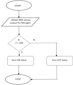
The dispensary system, microcontroller, and sensor system make up its three key components. Based on the findings of a soil test, the control system determines how much fertilizer needs to be added. Fertilizer is assessed based on the amount of nutrients present and added accordingly. The amount of fertilizer provided as a supplement to crops at different stages of their growth to maintain balance—that is, while the nutrient levels are within optimal ranges—is known as the maintenance dosage.
