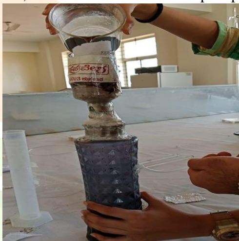
Fig. 6. Extraction of lignin
