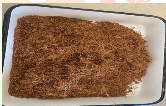
Fig. 3. Coconut coir in small pieces and kept in oven.
