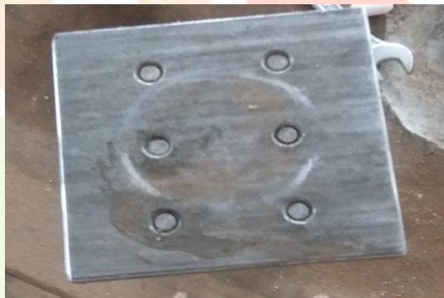
Figure 2: Piled raft arrangement for 4 number of piles
