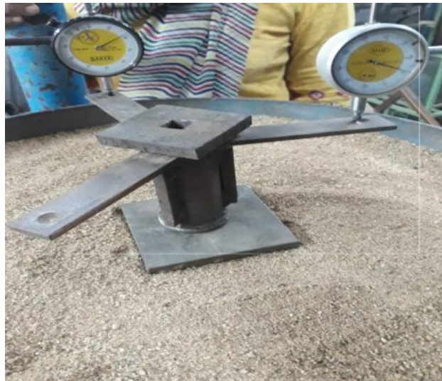
Figure 7: Model Test setup for plain raft foundation
