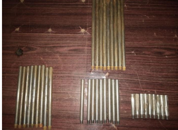
Figure 5: Model Steel Piles.
