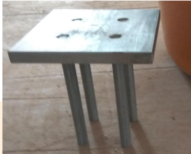
Figure 2: Piled raft arrangement for 4 number of piles
