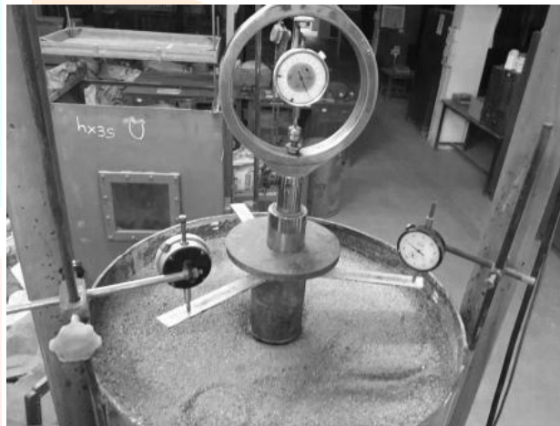
Figure 6: Model test set up with connector, proving ring and dial gauges
