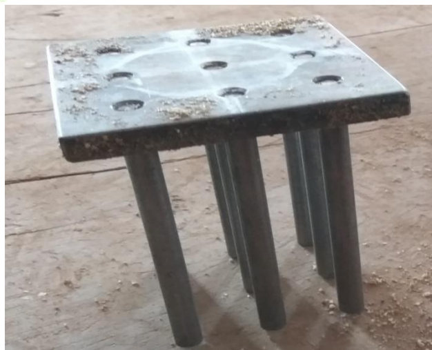
Figure 4: Piled raft arrangement for 9 number of piles
