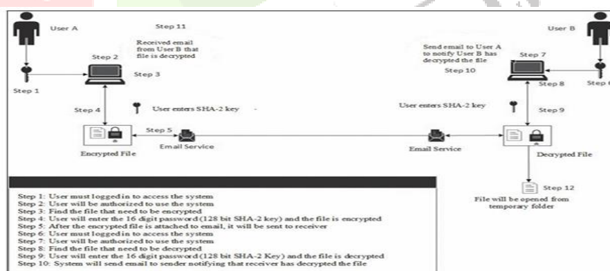
FIGURE 1. General Architecture of HES.
