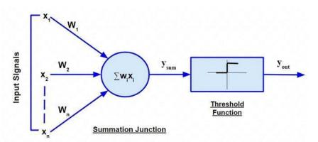
Simple McCulloch-Pitts neurons are capable of representing logical operations. To achieve this, the connection weights and the threshold function must be appropriately chosen.
