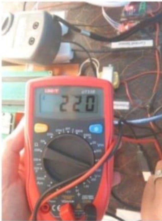
Fig. 11. Current and Voltage on DMM for 120W Load
