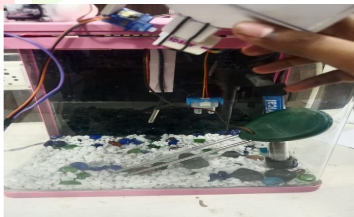
Fig 4 : Hardware setup front view
