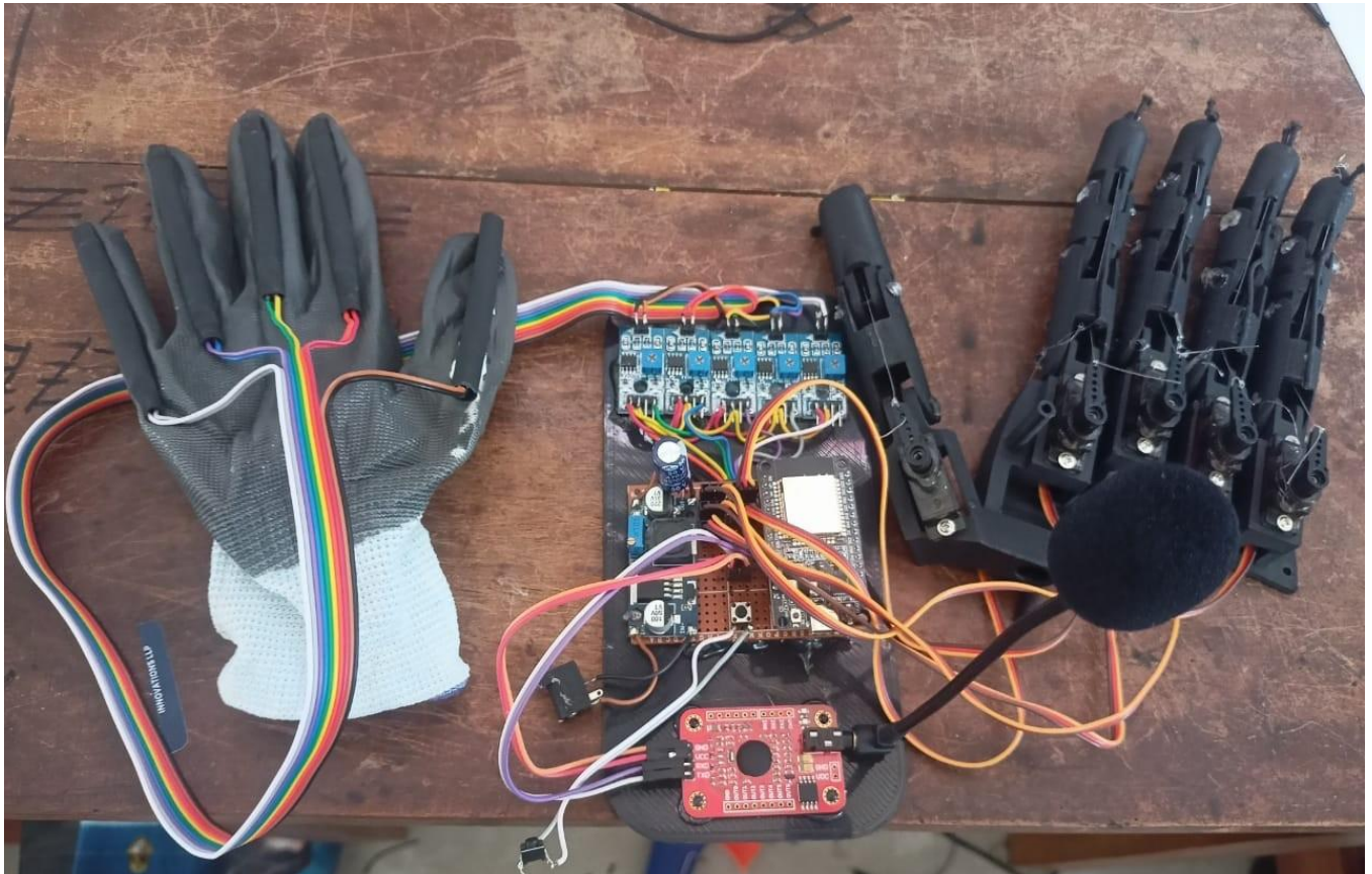
Fig. 4. Hardware prototype of the hybrid-controlled prosthetic finger system
