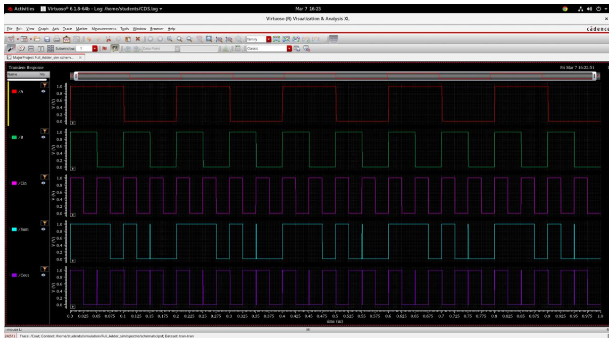
Fig. 4. Input/output transient waveforms and delay cursors.
