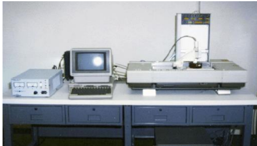
Figure 1.1: The Stereolithography Apparatus by Charles W. Hull
