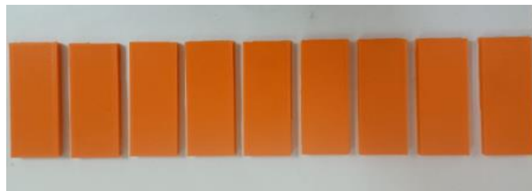
Fig.5 3D printed ABS Specimens according to the L9 Array
