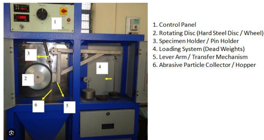
Fig.4 3-Body Abrasive Wear Testing Equipment
