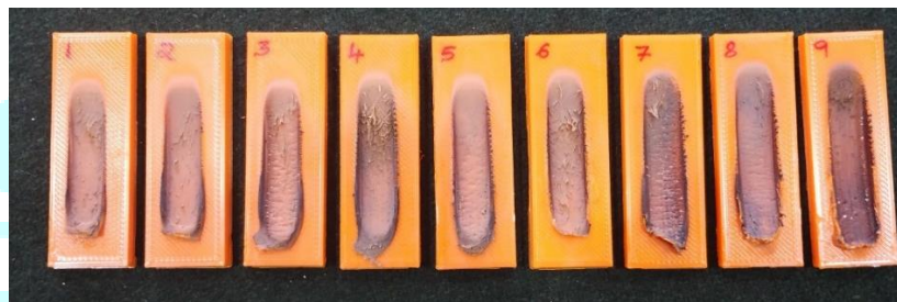
Fig.7 3D Printed ABS worn Specimens
