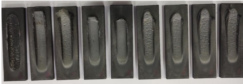
Fig.9 3D Printed ABS+CF worn Specimens
