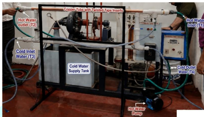
Figure 4. Experimental Set Up in Lab.
