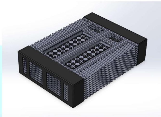
Fig. 10: Final CAD Model with Battery Cells
