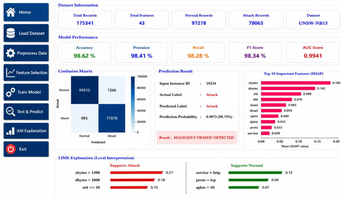
Figure 6.1 Intrusion detection system dashboard UI
