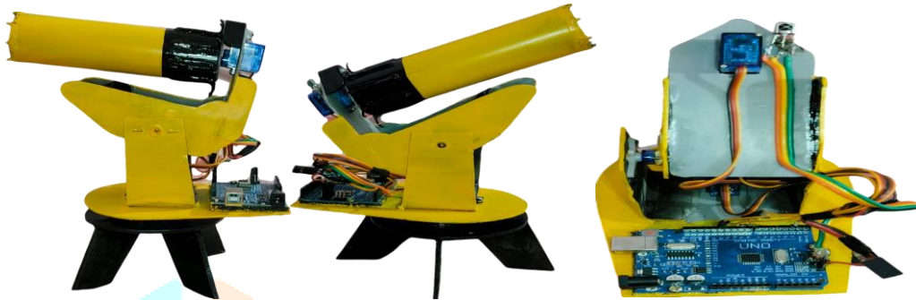
Figure 2: Overall System Architecture of Face Tracking IR Turret
