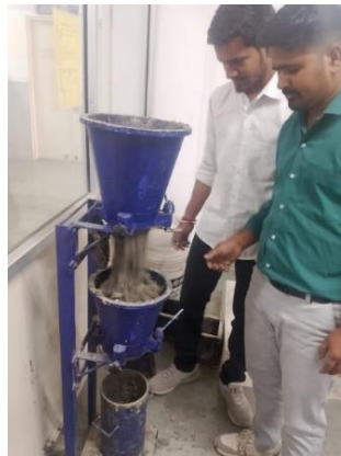
Figure 3: Compaction Factor test
