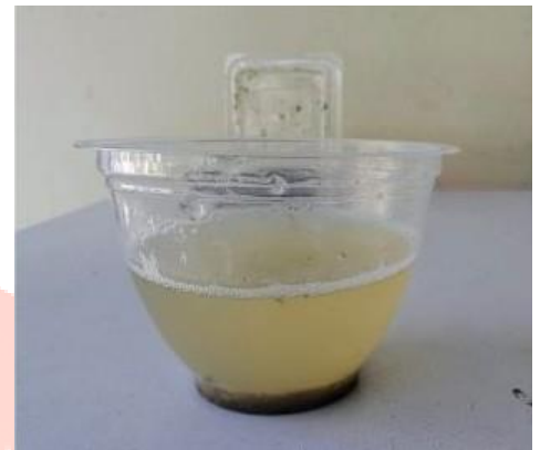
Figure 3.1.3: Biofilm samples on Day 3 — \alpha -cellulose film fully dissolved; starch film persisting.
