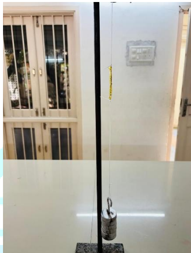
Figure 3.4.1: Vertical hanging test setup — biofilm strip (1 cm × 5 cm) clamped to stand with weights.
