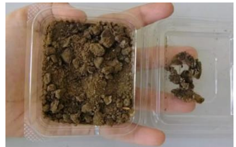
Figure 3.2.3: Biofilm disks after Day 3 — papaya leaf extract film fully degraded; others partially decomposed.
