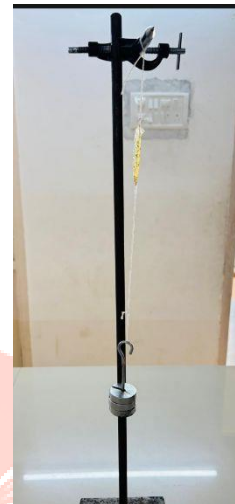
Figure 3.4.2: Vertical hanging test — biofilm strip at breaking point under applied mass.
