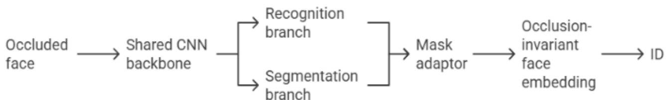
Figure 3: SOIDN architecture (Zeng et al. [11]) showing simultaneous recognition and segmentation branches connected by the occlusion mask adaptor module.
