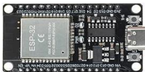
Figure 6.1: ESP32 Development Board
