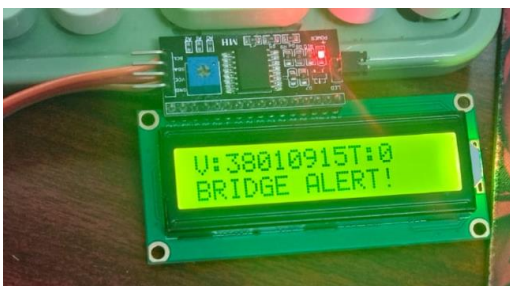
Fig.7 Bridge Alert output in LCD
