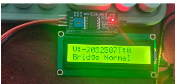
Fig.8 Bridge Normal output in LCD
