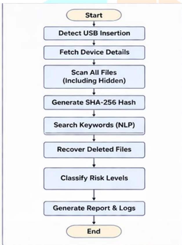
Fig. 1: System Architecture of USBGuard-AI Forensic Framework
