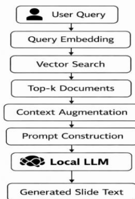
Fig. 2. Language model generation and document retrieval are integrated in the Retrieval-Augmented Generation pipeline.
